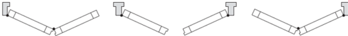
6 Panel Bi-Fold 2 Bi-Fold Panels Hinged Left, 2 Bi-Fold Panels Hinged Right, & 2 Panels Individually Hinged (1 Left & 1 Right) With 2 T Post "LLTLRTRR"
